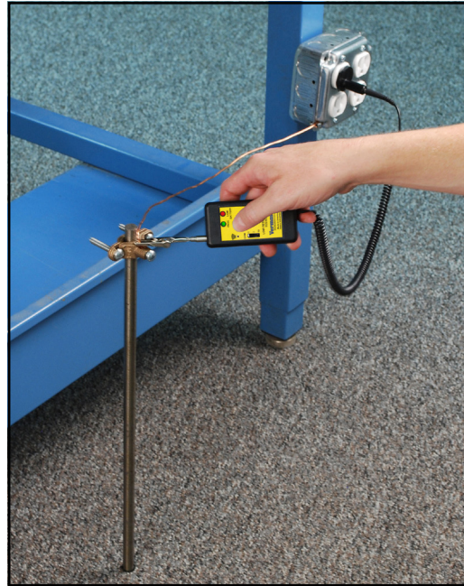
Figure 4. Testing auxiliary ground with the 222645 tester
