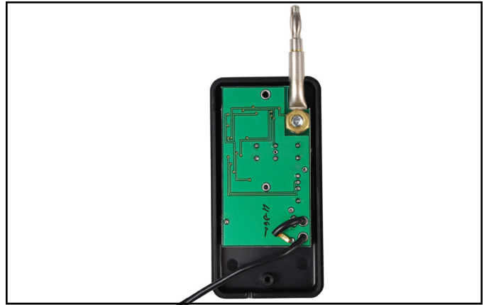
Figure 6. Removing the back cover
