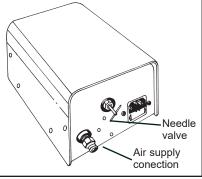
Figure 3. Airflow adjustment valve
