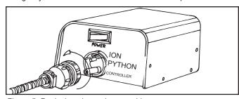
Figure 5. Replacing air nozzle assembly
