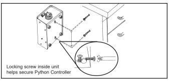
Figure 7. Installing controller to bench
