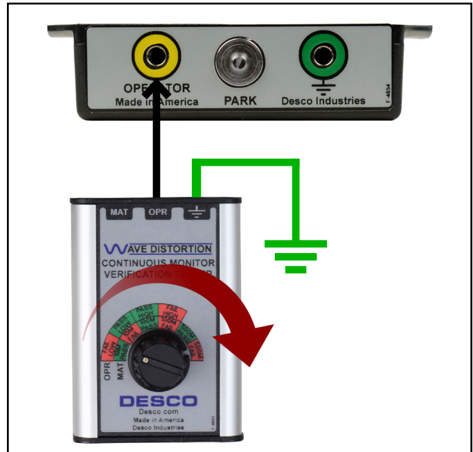
Figure 7. Connecting the Wave Distortion Monitor Verification Tester to the satellite remote's operator jack
