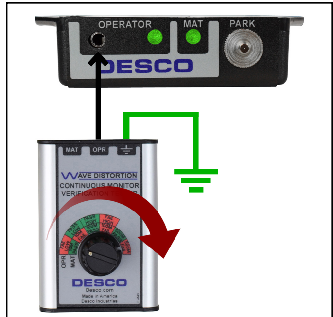
Figure 5. Connecting the Wave Distortion Monitor Verification Tester to the Mini Monitor's operator jack
