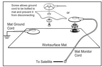
Figure 7. Installing the Mat Ground and Mat Monitor Cords
