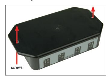
Figure 2. Mounting the Control Unit
