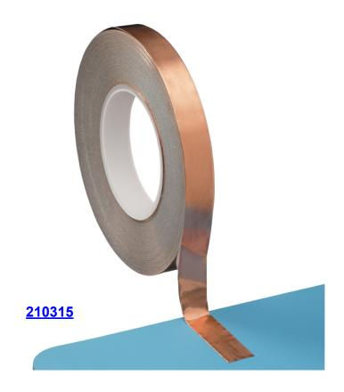
Copper earthing tape is used to ground ESD matting, polishes and paint. The tape is normally laid in strips 4 to 8 metres apart, across the full width of floor, under the floor covering, and then connected to earth protective ground.
